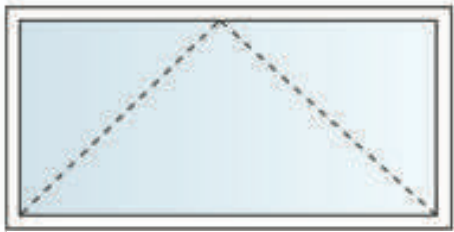
12 Top-hung outward opening awning window
